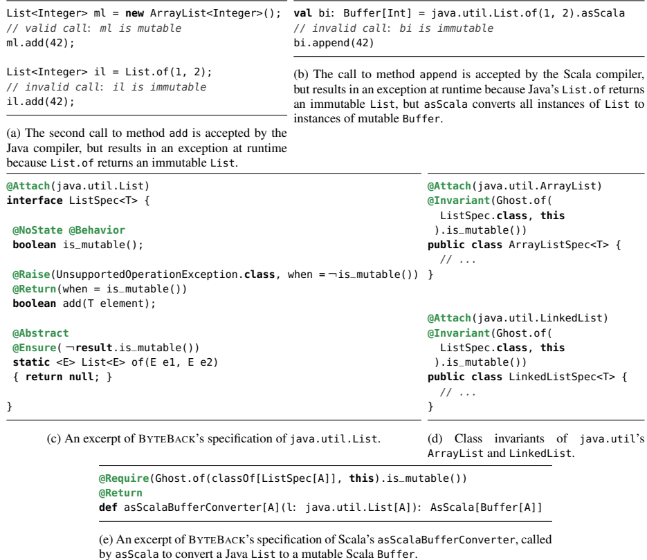
Fig. 1: An example of behavioral substitutability errors that are uncaught by the Java and Scala type systems, which can be precisely analyzed with this paper’s deductive verification technique. The annotations use a simplified BBLib syntax, similar to the one used in previous work on BYTEBACK [23,22].
